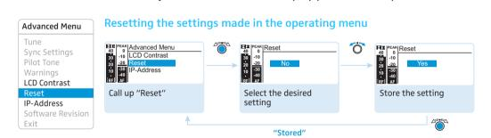
When resetting the settings made in the operating menu, only the selected settings for the pilot tone and for the frequency banks "U1" to "U6" remain unchanged. For an overview of the factory-preset default settings, refer to the supplied frequency information sheet.
